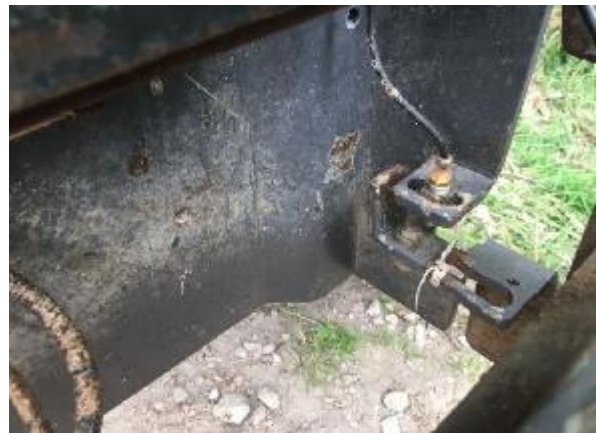
Front bar sensor will activate the emergency stop if the hinged bar makes contact with something and is pushed back
