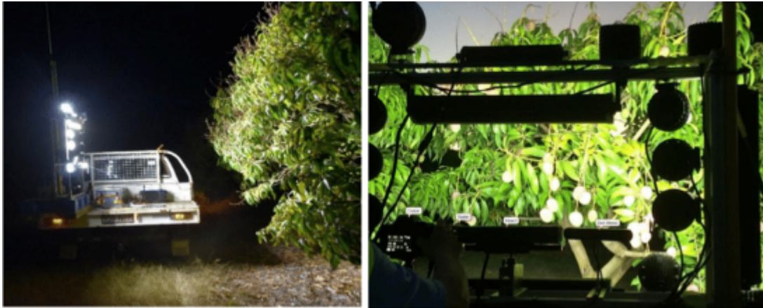
Central Queensland University Machine Vision imaging rig, operated at 6klm/hr
