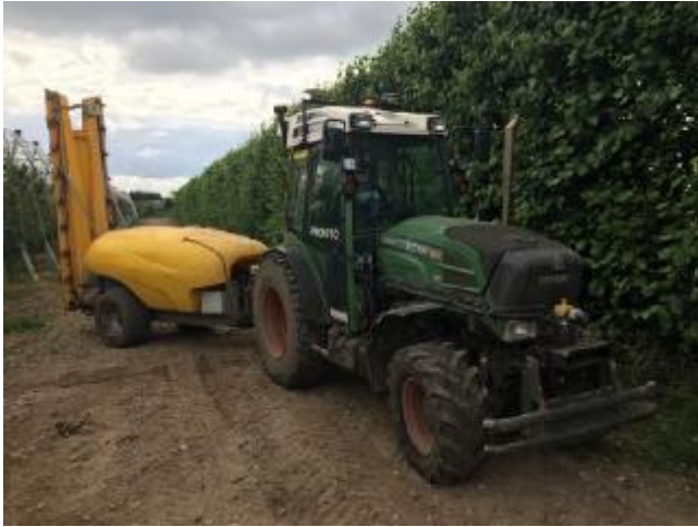
Verkooijen Fruits' Fendt 208V spray tractor fitted with Precision Makers Autonomous System
