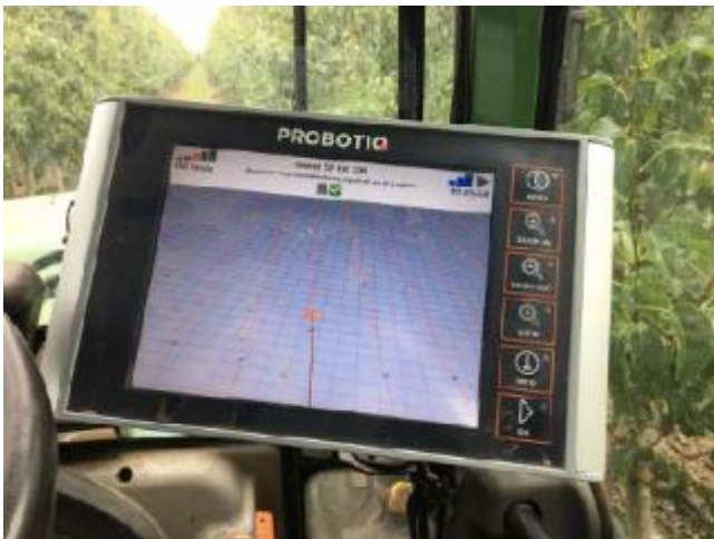
In-cab control system and navigation map.
