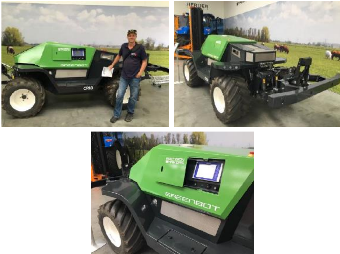
Figure 17: GreenBot, Precision Makers, NL, Standard 3-point lift, PTO, hydraulic remotes and GreenBot manual control centre, also controllable via the cloud [Source: Author]
