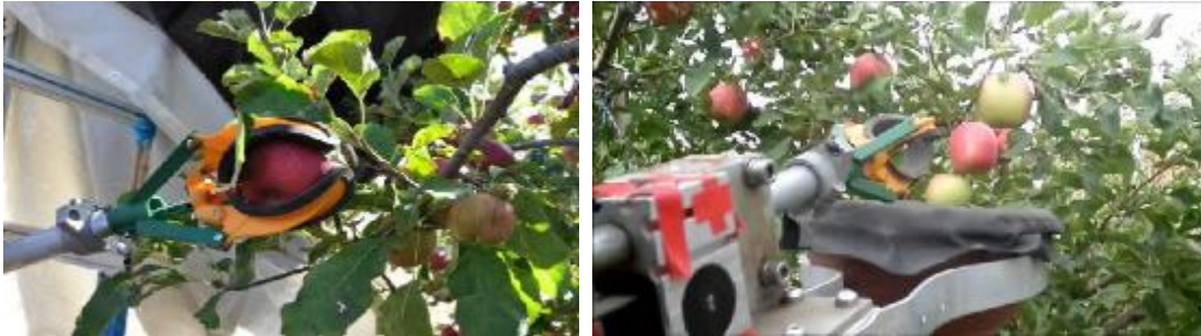
Figure 31: L-R: Fresh Fruit Robotics Israel apple picking 'grabber' and robotic harvest showing the 'drop bag' under the picking hand [Source: Gad Kober]
