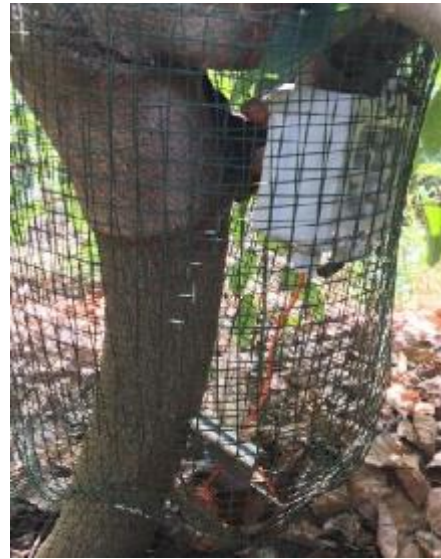
Wireless 'dendrometer' measuring trunk diameter variations due to moisture stress, Israel
