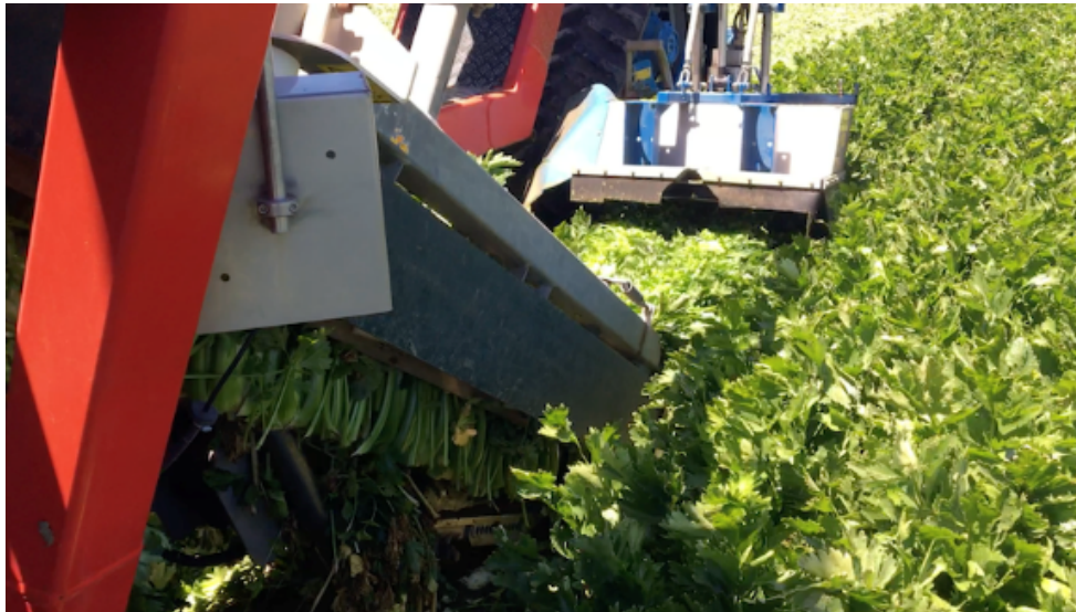
Figure 21: Leafy tops are removed at an exact height, then the crop is ‘cut’ from the ground using high pressure water, then ‘grabbed between two rubber belts and elevated to the workers to clean and pack [Source: Author]
