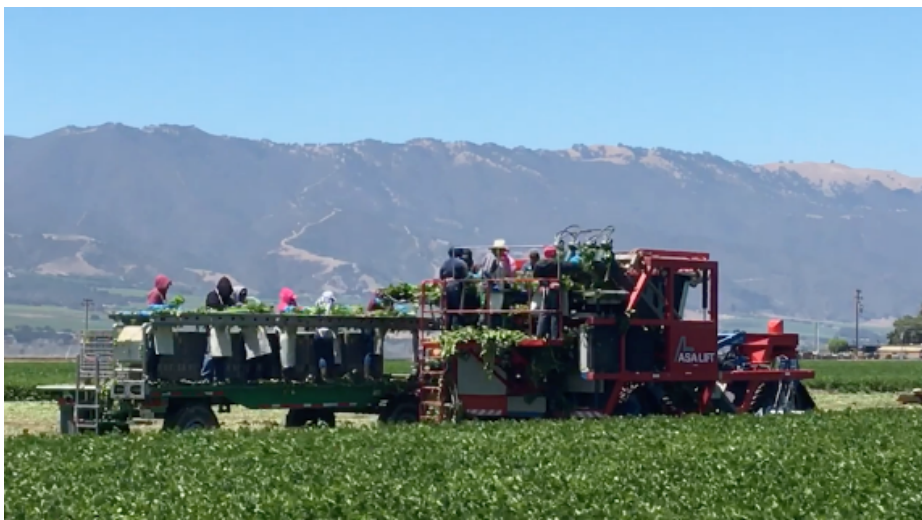
Figure 22: All workers are at a comfortable standing height. Ten workers can cover the same area as up to 50 ‘hand harvesters’ [Source: Author]
