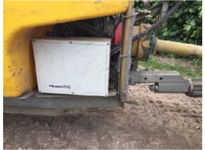
The 'smart box' required on the sprayer to communicate with the in-cab control system.
