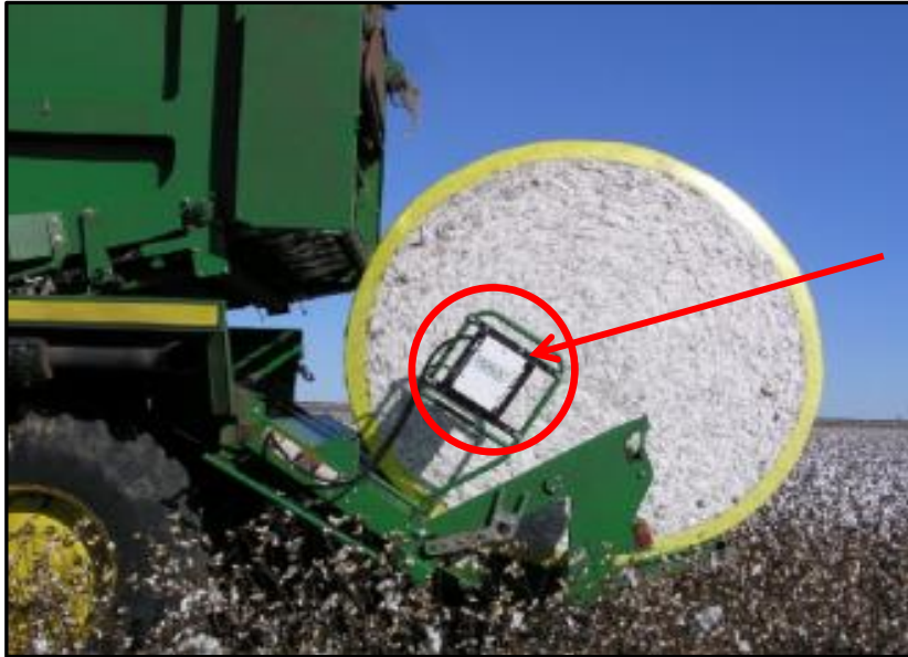
Figure 7: An on-board moisture meter fitted to a round module picker.
