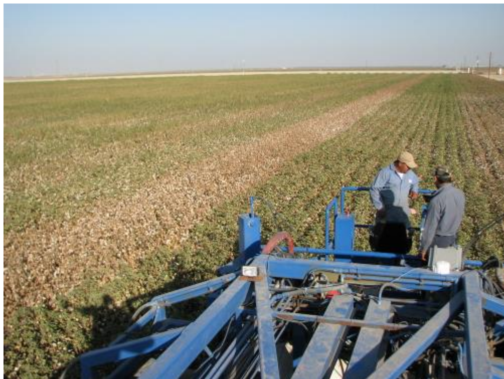
Figure 12: Commercial thermal defoliation unit that treats 6 rows per pass. The rows on the left were treated 12 hours before and are easily visible.
