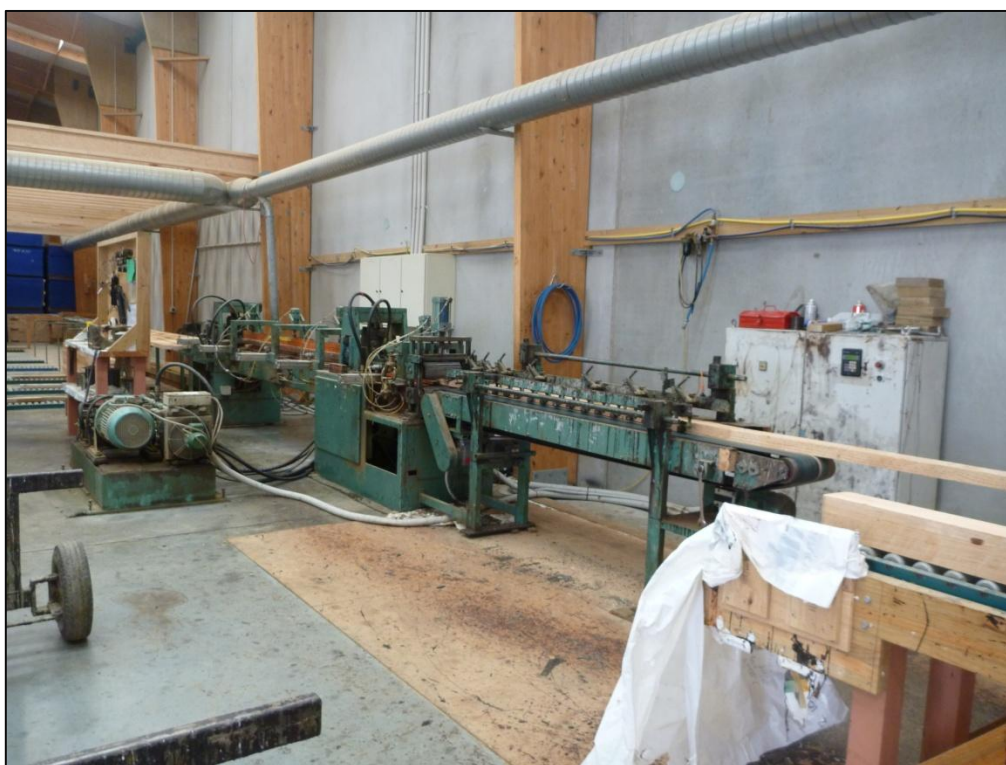
Second hand basic small-scale European finger jointer, manual feed and gluing at Timberbond
