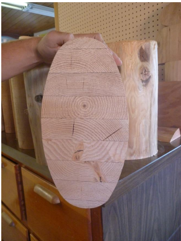
Laminated and turned Douglas fir pole from Pacific Timber. Growth rings of 2nd and 3rd growth plantation Douglas fir are not dissimilar to achievable growth rates in England
