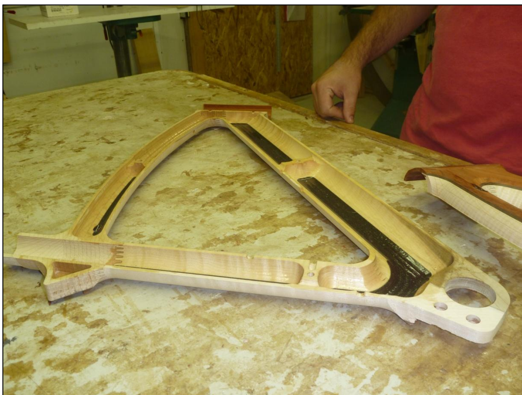
Complete routing and finger jointing used to create lightweight structurally efficient bike frames from hardwood timber
