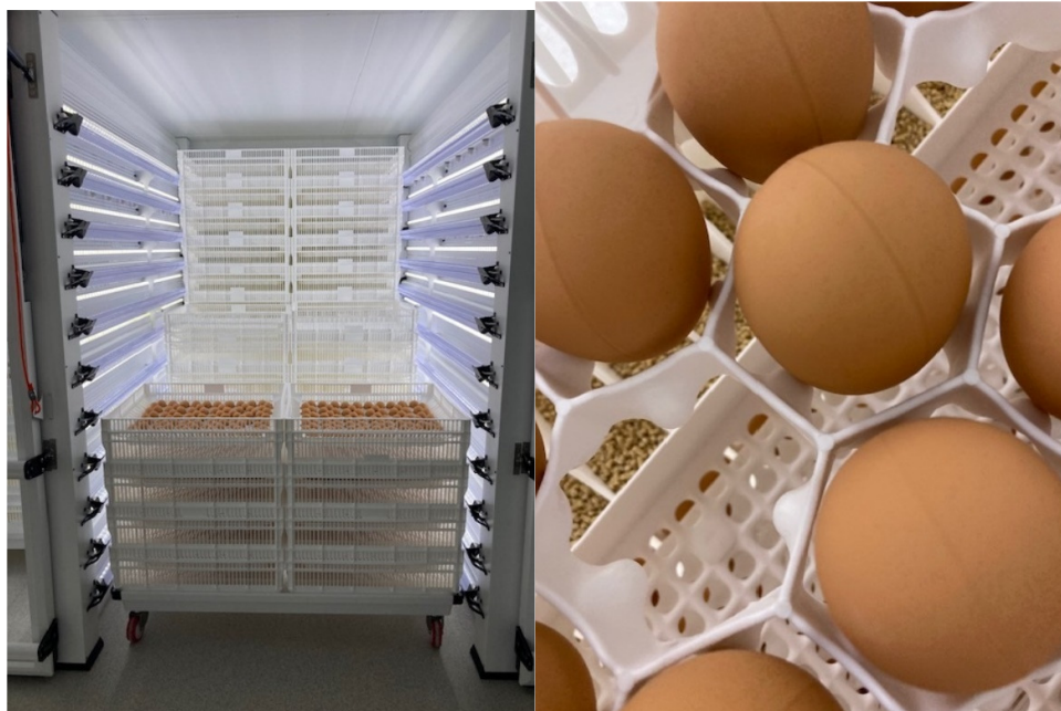
Fig 18 – the HatchTech HatchCare system showing the trays and their access to feed and water
