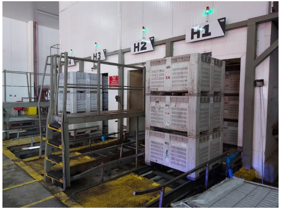
Figure 4 : Cherry bin in arrival hall about to enter a hydrocooler in Garcés, Chile. Photo: Author's own.
