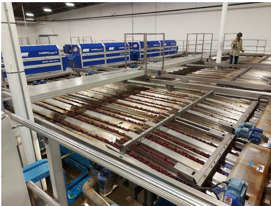
Figure 7: Unitec Cherry Vision 48 lane Sorting System at The Dalles Fruit Company, US. Photo: Author's own.
