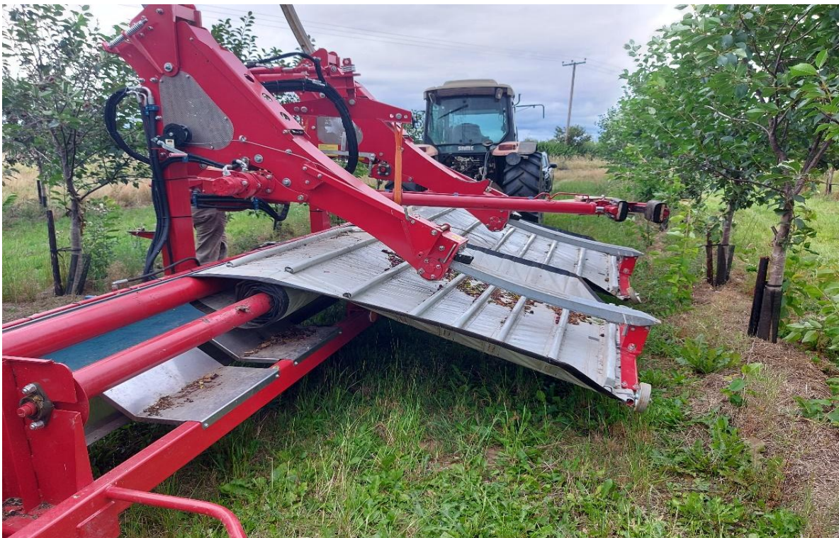
Figure9: Weremczuk Shake and Catch, sour cherry harvester, Herefordshire, UK. Photo: Author's own.
