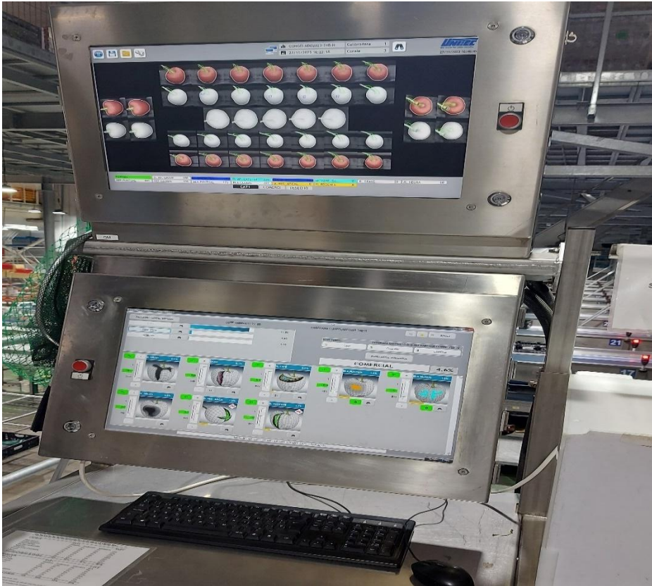
Figure 7: Unitec Cherry Vision 3, Control Computer for Defect Scanner at Garces, Chile. Photo: Author's own.
