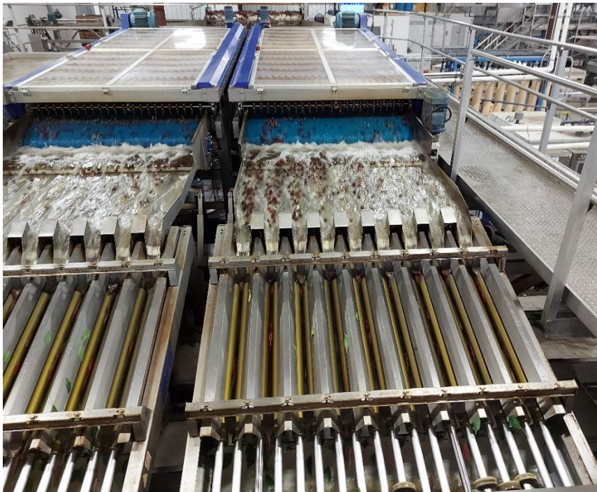
Photo 6: Unitec cluster cutter at The Dalles Fruit Company, US. Photo: Author's own.
