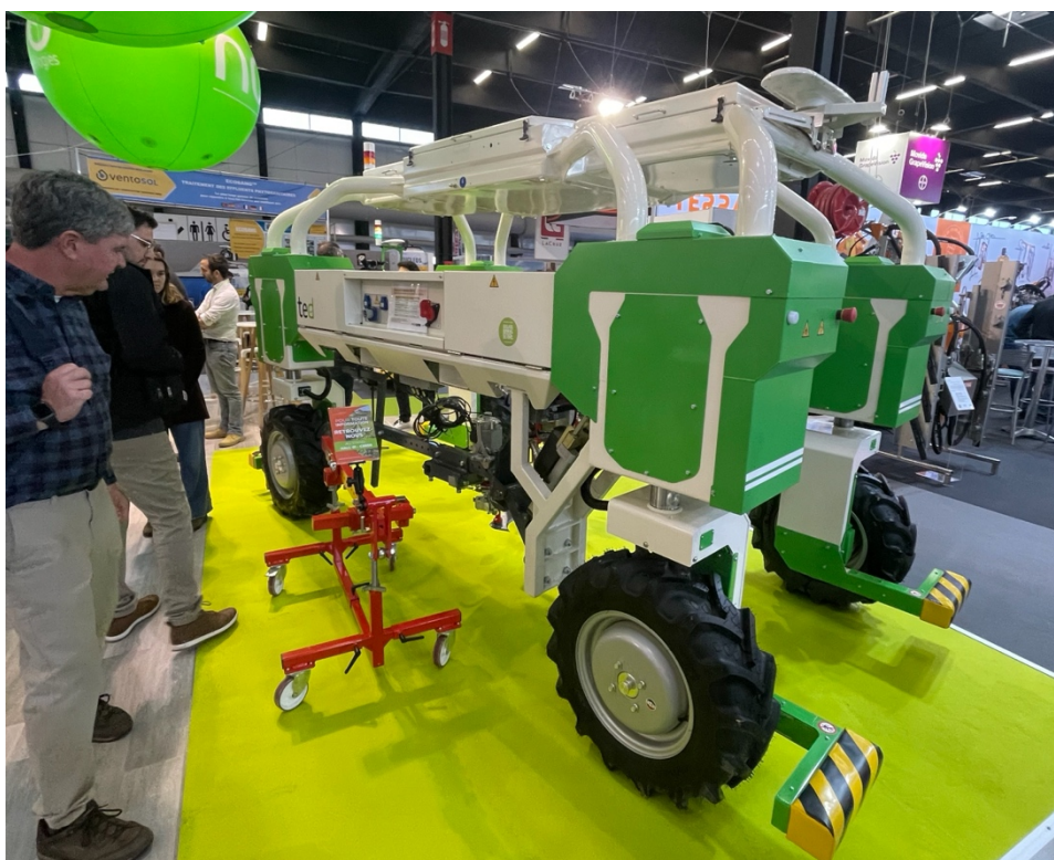
Figure 14 Demonstration of 'Ted' Autonomous Vineyard Robot by Naïo Technologies tool designed specifically for vineyard maintenance. Its primary function is to perform precise mechanical weeding between vine rows, offering an eco-friendly alternative to herbicides and promoting sustainable viticulture practices.
