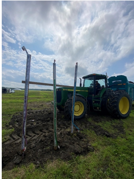
Figure 7: Effect of tyre pressure on soil compaction, Training for farmers in Canada. (Source: Author)
