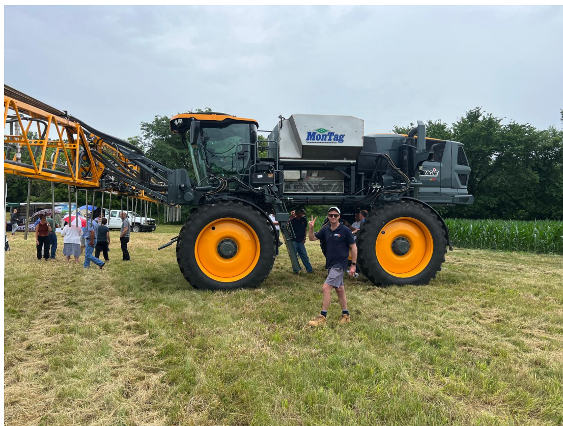
Figure 22 A custom built cover crop seeding machine, adapted to a high clearance sprayer to seed cover crops in growing corn crops in Iowa USA, featuring impressed fellow scholar Billy Browning at a Heatland Co-Op field day in July 2022, near West Des Moines Iowa. (Source: Author)
