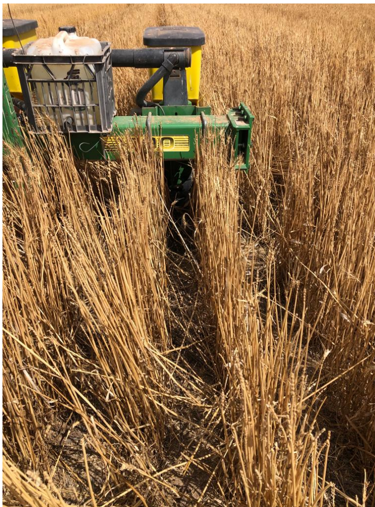
Figure 20 Semi irrigated cotton being planted behind stripped wheat, highlighting the importance RTK GPS for effective inter-row sowing, and ability of disc planters to plant through high residue situations. (Source: Author)
