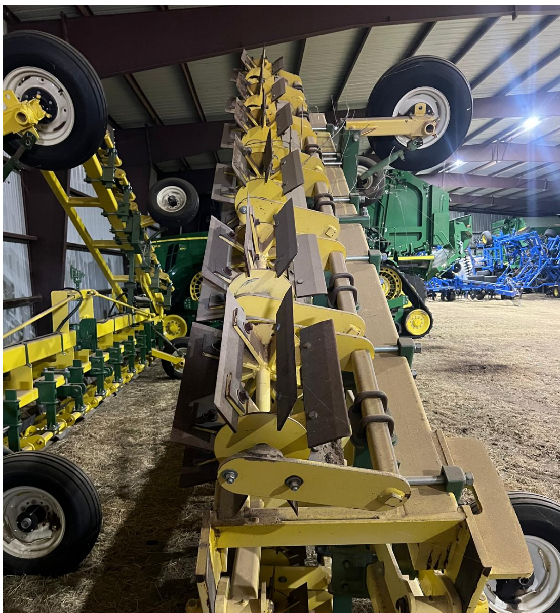
Figure 21 a stalk chopper at lance and Danielle Williams Panhandle TX USA used to destroy old crop rows while retaining crop residue on the soil surface. (Source: Author)
