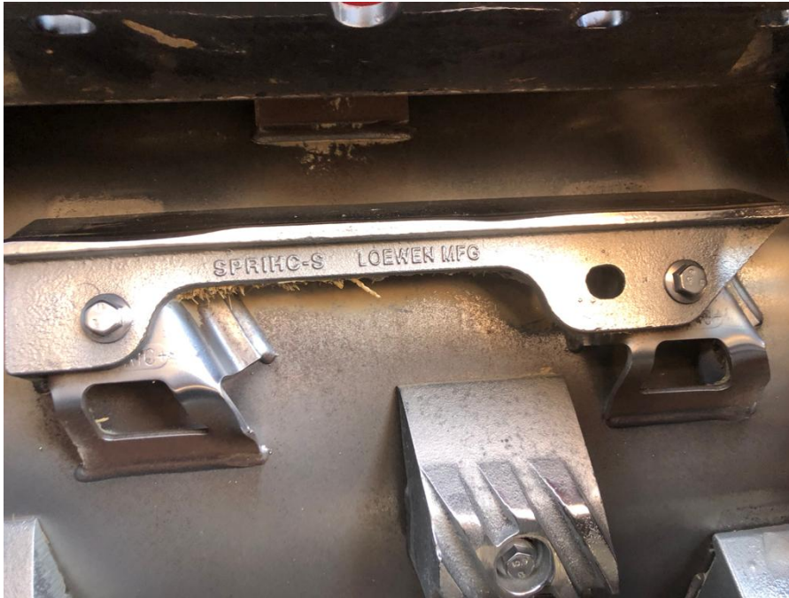
Figure 6 Modifications to a Case IH Flagship rotor threshing elements, including straight separator bars and 10° rasp bars (Source: Author)
