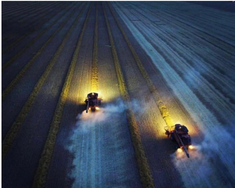
Figure 1 Poor spread pattern of factory residue spreaders, showing the uneven distribution of plant material across the swath width. (Source: Rhylie Botheras)
