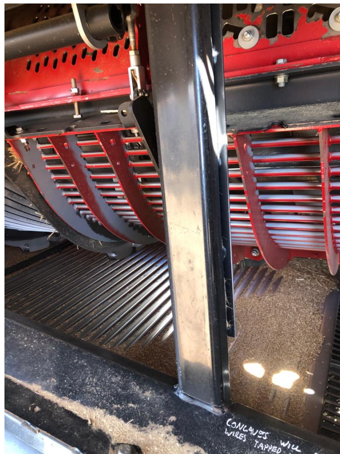
Figure 7 Case IH Flagship Combine LHS rotor with hard thresh helical concave in Position 1, and round bar concaves in Position 2, 3 and 4, with paint removed from grain separation in Position 2 round bar concave after only one season (Source: Author)
