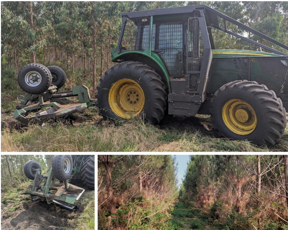
Figure 19. Rouleau landaus machine clearing inter row vegetation, France. Source: Author's own.
