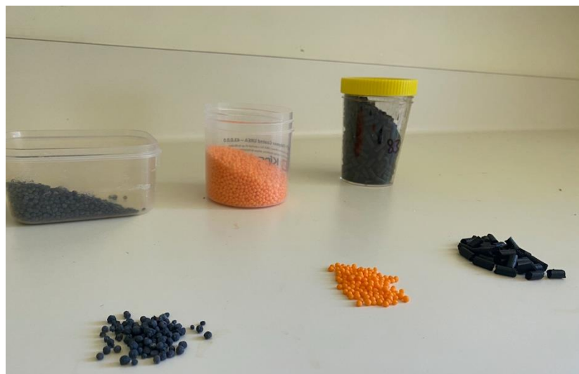
Figure 4: Biochar coated urea, poly coated urea, pelletised Oat biochar with urea (Author's own)
