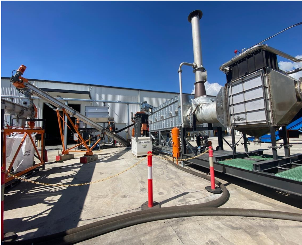
Figure 13: Large scale production with Pyrocal's commercial pilot plant in Toowoomba, QLD (Author's own)
