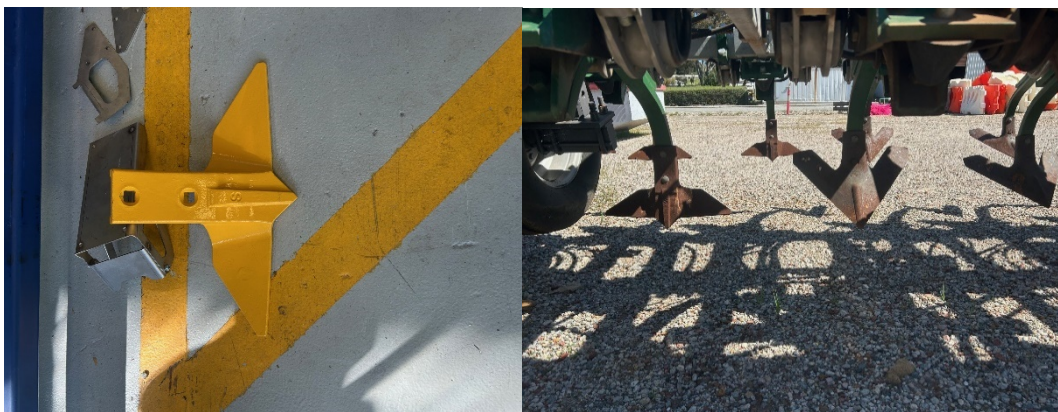
Figure 4: New point design (source: author) Figure 5 Point Comparison New Vs Old (source: author)
