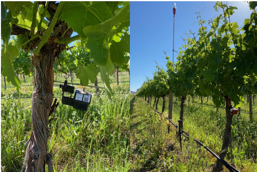
Figure 6 – Dendrometer location on vine pictured left, and three Dendrometers alongside a soil moisture monitoring probe in Bleasdale Vineyards pictured right (Source: Author, 2021)
