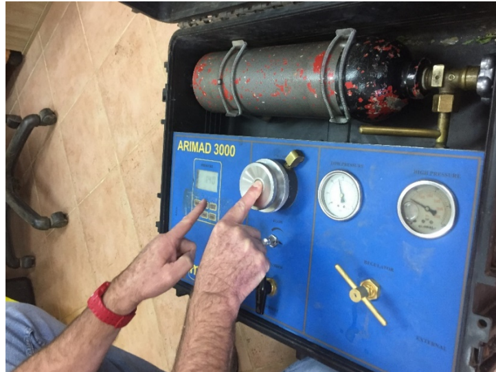
Figure 10 - Netafim uses a pressure chamber to measure stem water potential in their company vineyards, 2019 (Source: Author, 2019)
