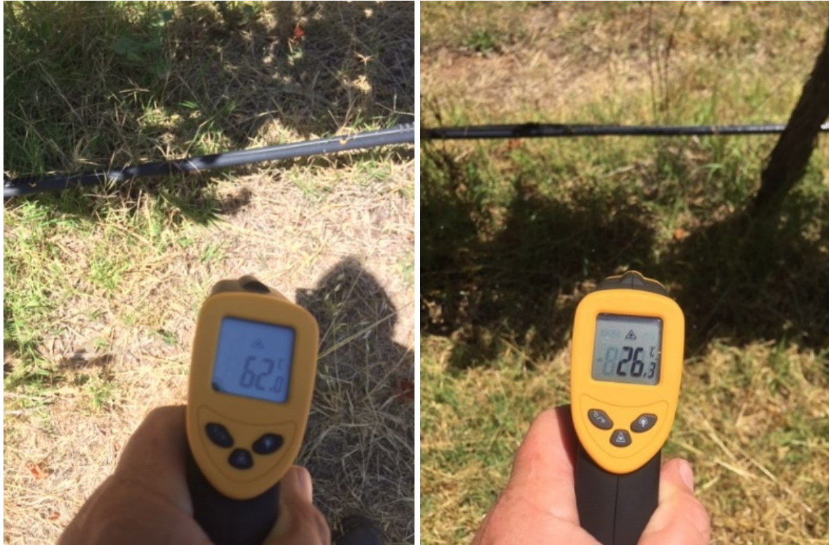
Figure 23 - Left, infrared temperature on bare ground undervine compared to the temperature of undervine with actively growing ground cover, 30th January 2020, 39°C (Author, 2020)
