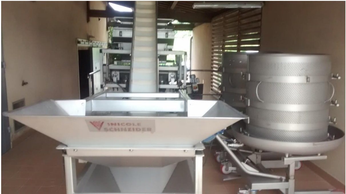
Figure 5: Modern equipment depicting a hopper leading to an elevated crusher (Source: Author)
